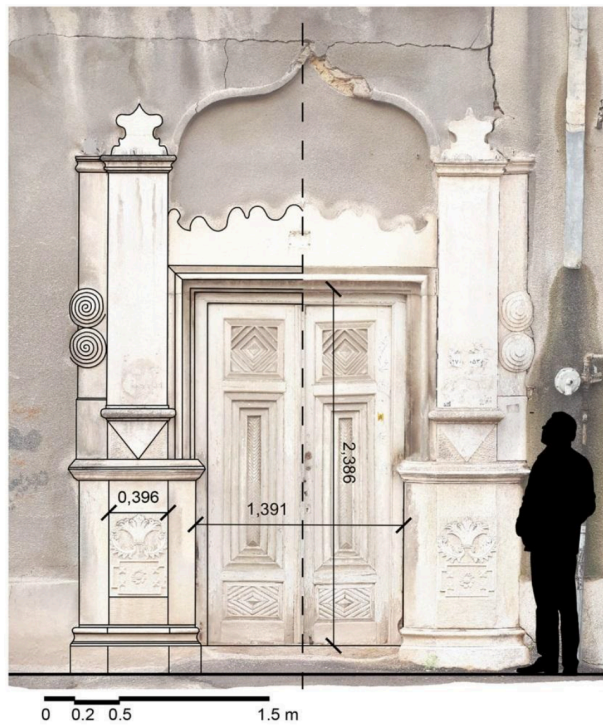
Fig.4. Drawing on the final metric orthoimage in AutoCAD
